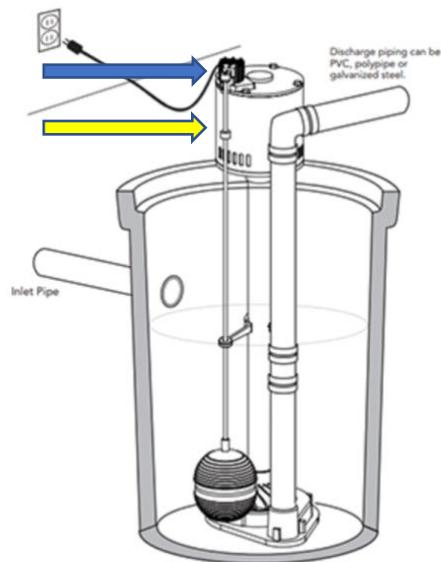
Above - is a pedestal pump. On the float shaft the Blue arrow shows the adjustment for turning the pump OFF. The Yellow arrow shows adjustment for turning the pump ON as the float rises
