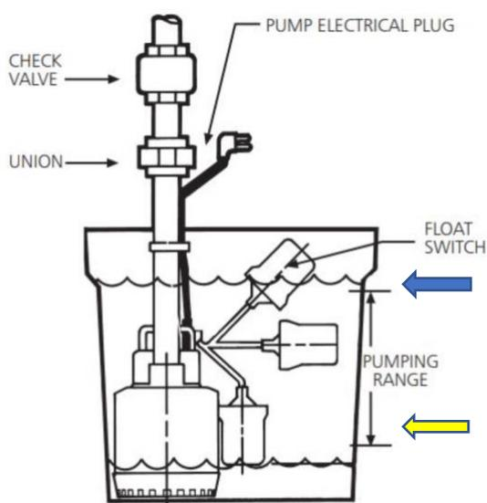
Above - is a submersible sump pump. The Blue arrow shows water level where the sump turns ON. The Yellow shows the water level where the sump turns OFF.
